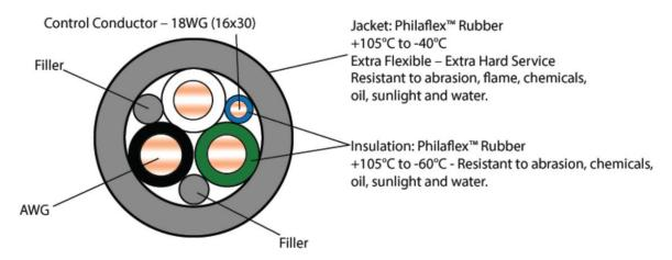
Figure 1: Cross section of Philatron Philaflex EV charging cable. Source: Philatron
